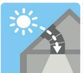
The **rigid** tunnel is ideal for distances between roof and ceiling from 0.9 to  $1.7\ m$  - with extension sections up to 6 m.
